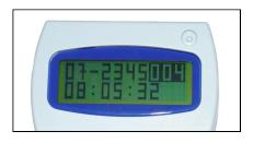
By pressing the <OK> button the screen display will alternate between a large sized print display and a smaller sized but more detailed print display.
