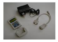
• A Speedy pack contains: Speedy with holder, one loft-antenna and a power supply (12V) with adapter-cable.
