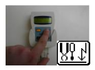
• Antenna test: to test the detection quality of the antennas. Press "OK". Speedy will mention the number of antennas found. When you hold some rings over the antennas, Speedy will start beeping. This allows you to see if the antenna installation is done properly, and if the registration quality is good. Speedy should already beep if the chip-ring is held on a height of 5 to 6 cm (2 to 3 inches)
