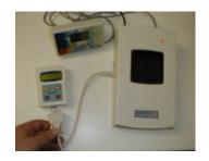
PC- Connection: Speedy is connected to a PC via a special converter with modem-cable. Via a split-cable (Y) the clubantenna is also connected. Attention, you may only connect Speedy if the PC gives you the command to connect the clock.
